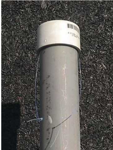
Fig. 19. Cap on antenna pipe to keep rain out and to trap fishing line holding the antenna
