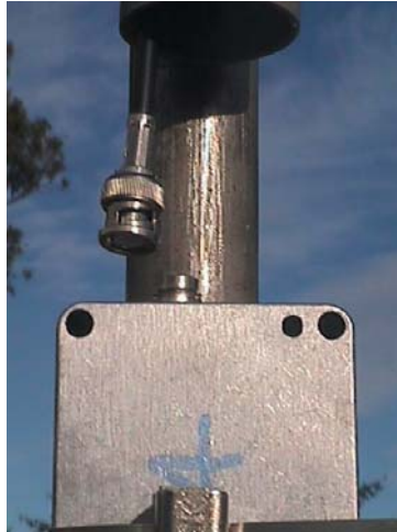
Fig.20. Preamplifier slid down to allow antenna BNC connection to preamplifier BNC
