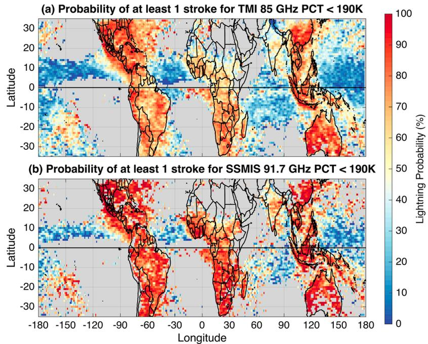
**Figure 8.** (a) Probability of at least one lightning stroke given TMI 85 GHz PCT below 190 K. (b) Probability of at least one lightning stroke given SSMIS 91.7 GHz PCT below 190 K.
