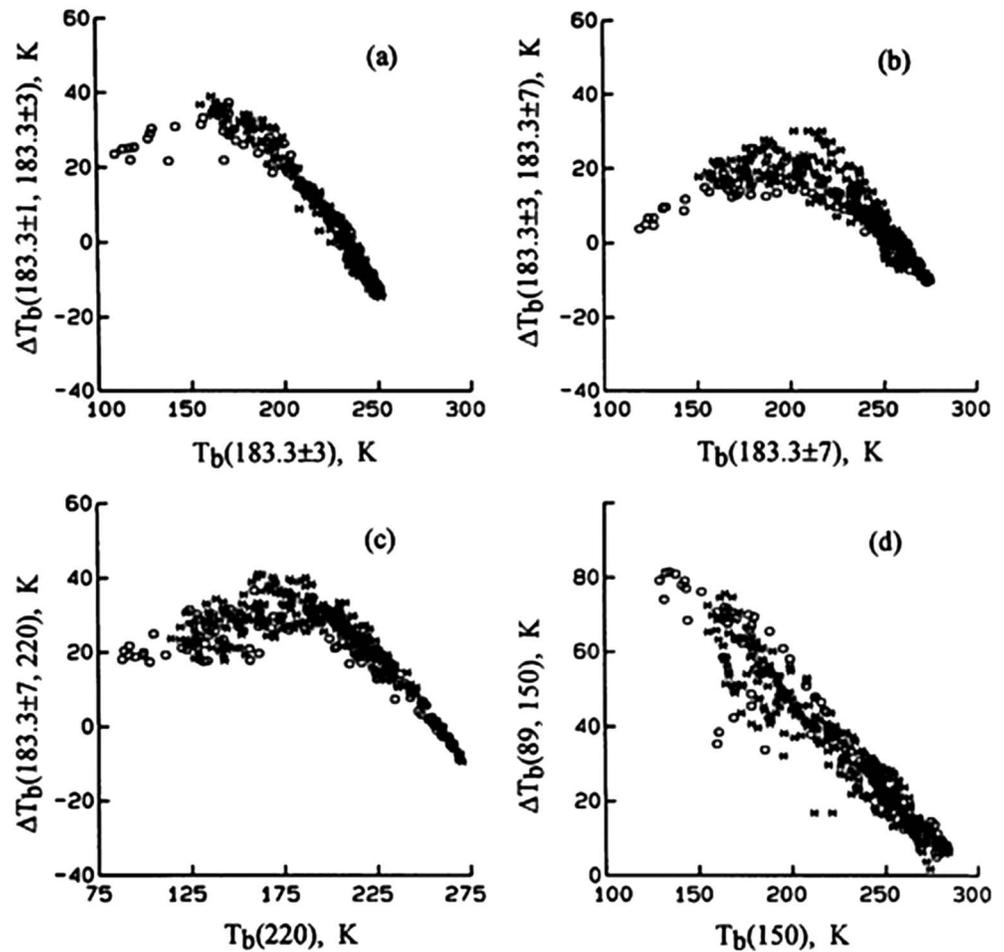
**Figure 1.** Reproduction of Wang *et al.* [1997, Figure 11]. The scatterplot of  $\Delta T_b$ s and  $T_b$ s from pairs of microwave channels on an airborne radiometer for two storms. (a)  $\Delta T_b$ 13 versus  $183.3 \pm 3$  GHz, (b)  $\Delta T_b$ 37 versus  $183.3 \pm 7$  GHz, (c)  $\Delta T_b$  ( $183.3 \pm 7$ –220 GHz) versus 220 GHz, and (d)  $\Delta T_b$ (89–150 GHz) versus 150 GHz.
