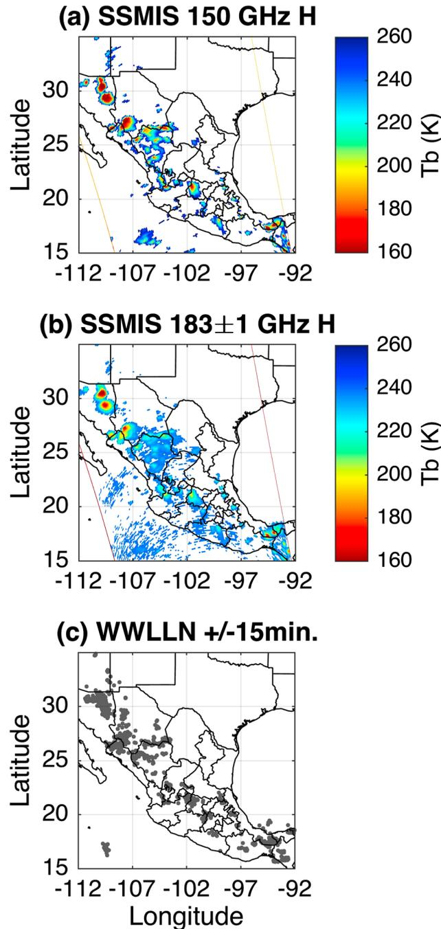
**Figure 14.** SSMIS-F16/WWLLN case study over Mexico at ~1900 LT, 14 August 2010. (a) SSMIS 150 GHz H data and (b) SSMIS 183.3 ± 1 GHz H data. (c) Lightning strokes (gray dots) for ±15 min of SSMIS pass time.
