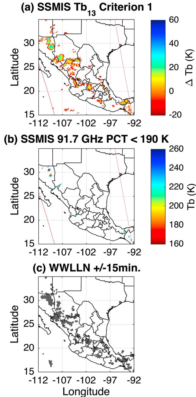
**Figure 15.** SSMIS-F16/WWLLN case study over Mexico at ~1900 LT, 14 August 2010. (a)  $\Delta T_{13}$  for 183.3 GHz  $T_b$ s that satisfy criterion 1 in section 2 from Hong and Heygster [2008] and (b) SSMIS 91.7 GHz PCT data below 190 K. (c) Lightning strokes (gray dots) for  $\pm 15$  min of SSMIS pass time.
