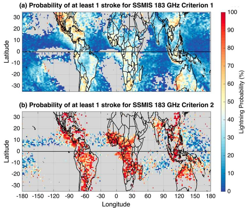
**Figure 7.** (a) Probability of at least one WWLLN lightning stroke given criterion 1 in *Hong and Heygster* [2008] for deep convection using SSMIS 183.3 GHz channels. (b) Probability of at least one WWLLN lightning stroke given criteria 1 and 2 in *Hong and Heygster* [2008] for deep convection using SSMIS 183.3 GHz channels.
