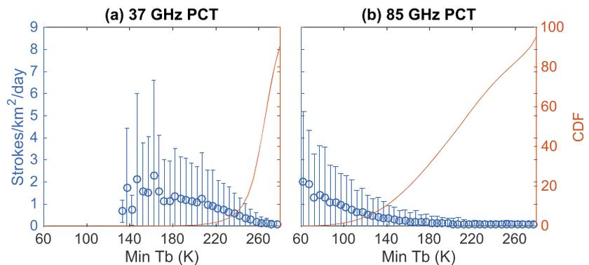
**Figure 3.** Scatterplot of TMI (a) 37 and (b) 85 GHz PCT brightness temperatures (Tbs) and WWLLN stroke rates. Similar to Figure 2 except that here blue circles are the averages of stroke rates within the Tb bins, and the error bars are the standard deviations of the stroke rates. Cumulative distribution functions (CDFs) of Tbs are shown on the right ordinate in red.
