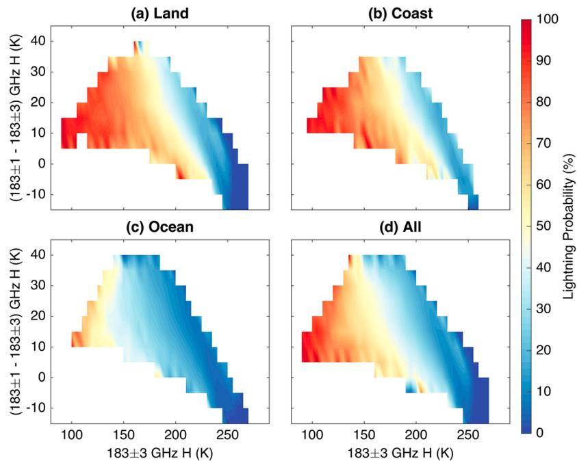
**Figure 12.** SSMIS  $\Delta T_{b13}$  versus  $183.3 \pm 3$  GHz H and probabilities of at least one WWLLN lightning stroke. Compare with Figure 1a that shows results from Wang et al. [1997].
