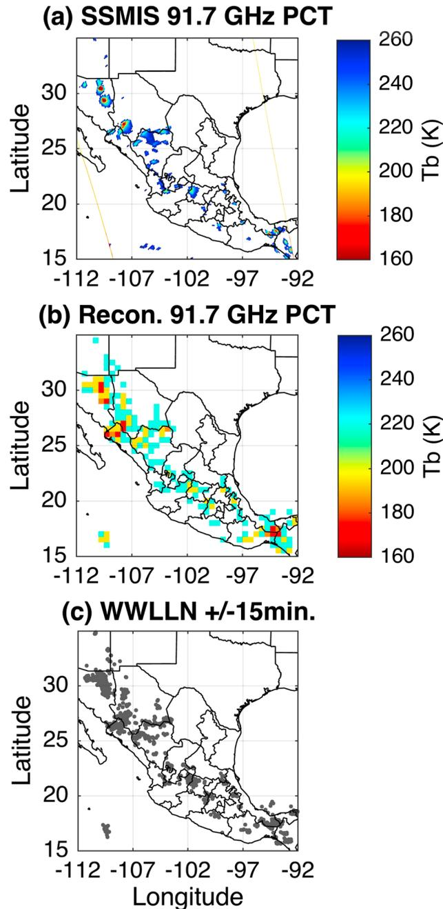
**Figure 13.** SSMIS-F16/WWLLN case study over Mexico at ~1900 LT, 14 August 2010. (a) SSMIS 91.7 GHz PCT data. (b) Reconstructed 91.7 GHz PCT data from WWLLN stroke rates and using scatterplots results in section 3. (c) Lightning strokes (gray dots) for ±15 min of SSMIS pass time.
