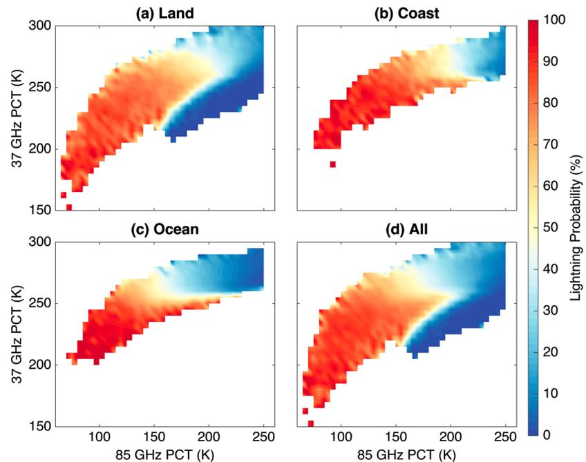
**Figure 9.** TMI 37 versus 85 GHz PCT and probabilities of at least one WWLLN lightning stroke.
